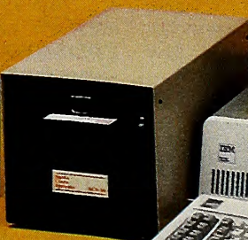
Shown below: 5MByte 5¼" hard disk with floppy backup.
