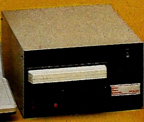
Shown below: Removable 8" 10 MByte Winchester cartridge drive.
